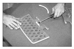
**Figure 8.20** Remove warming shelves and hardware from packaging. Install leveling bolt to each warming shelf.
